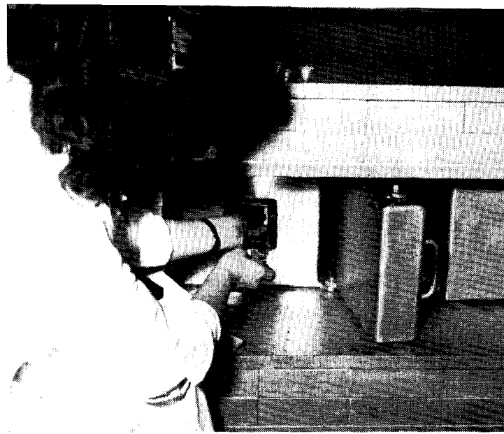
Technician at AEC's Health and Safety Laboratory inserts strontium-90 samples into low-level, anticoincidence counter
